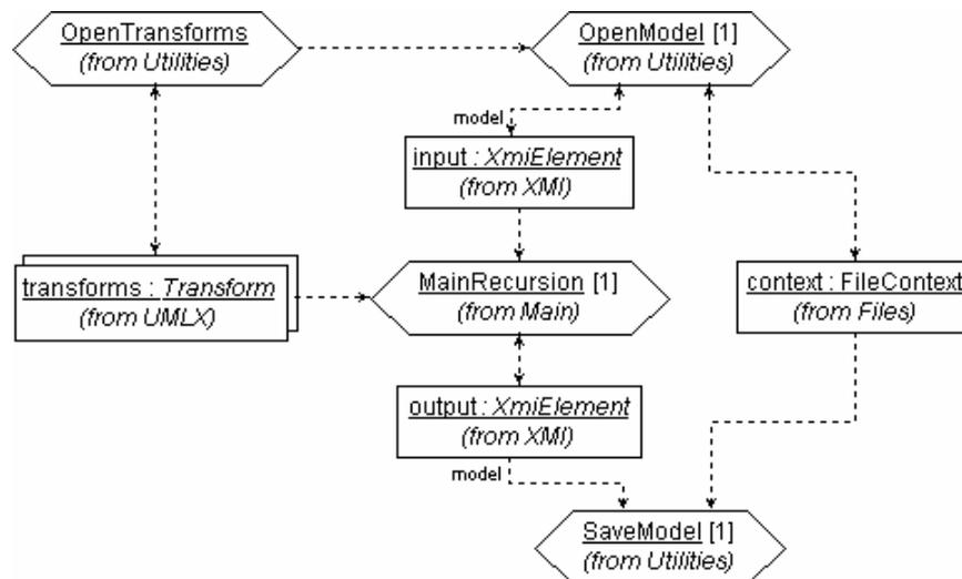
The main transform invokes `OpenTransforms` to identify the libraries of available transforms and then `OpenModel` to acquire the model which is then processed by the `MainRecursion`, whose result together with the context of the `OpenModel` is passed to the `SaveModel` prompter.
