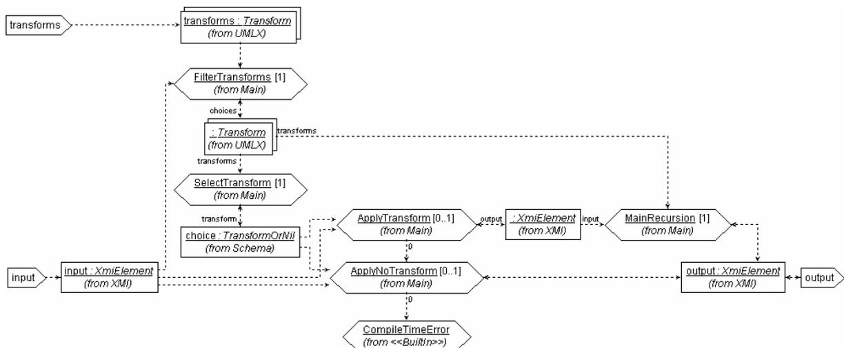
The `MainRecursion` first invokes `FilterTransforms` to identify the subset of the transforms that are applicable to the input, and then invokes `SelectTransform` to obtain an interactive choice of none or one transform. This choice is then passed to `ApplyTransform` and `ApplyNoTransform`. If `ApplyTransform` is successful its output is passed to `MainRecursion` for further activity. If `ApplyTransform` is unsuccessful `ApplyNoTransform` provides the result and the recursion terminates.
