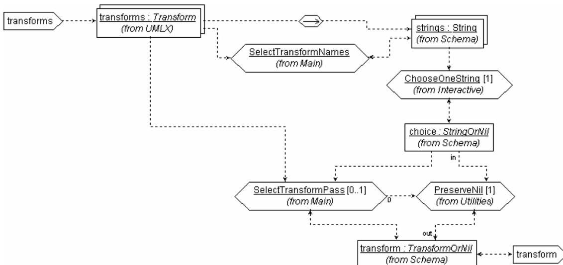
The collection of `transforms` is converted to a collection of `strings` for use by the `ChooseOneString` interactive transform. The chosen string or `Nil` is then passed to `SelectTransformPass` which identifies the chosen transform for return, or to `PreserveNil` which ensures a `Nil` return.
