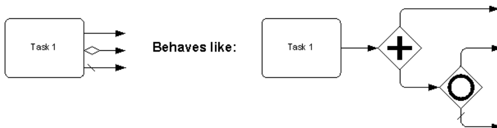
Figure 14-1 – Behavior of multiple outgoing sequence flow of an Activity
