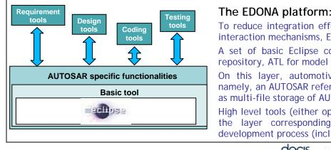
**The EDONA platform:** *A layered architecture based on Eclipse* To reduce integration efforts and harmonize modelling features and interaction mechanisms, EDONA is built upon Eclipse.
